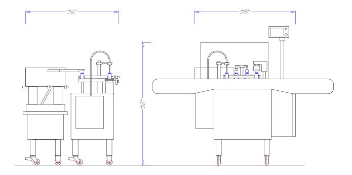
Width=965 mm, Depth=914 mm, Height=1320 mm, Weight: 1000 Newtons
